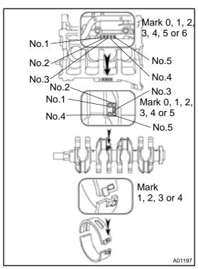
(m) If using a standard bearing, replace it with one having the same number. If the number of the bearing cannot be determined, select the correct bearing by adding together the numbers imprinted on the cylinder block and crankshaft, then selecting the bearing with the same number as the total. There are 4 sizes of standard bearings, marked "1", "2", "3" and "4" accordingly.
