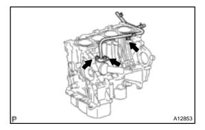
3. REMOVE WATER BYPASS PIPE
