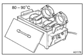
(b) Gradually heat the piston to  $80 - 90^{\circ}$ C (176 - 194°F).
