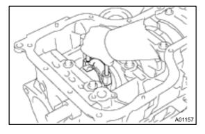
(c) Using the 2 removed connecting rod cap bolts, remove the connecting rod cap and lower bearing by wiggling the connecting rod cap right and left.
