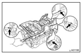
(c) Using a screwdriver, remove the bearing cap subassembly by prying the portions between the cylinder block and bearing cap subassembly. Remove the 5 lower main bearings.
