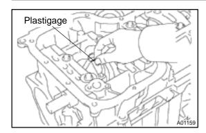
(f) Lay a strip of Plastigage on the crank pin.
