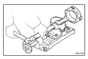
(c) Using a plastic–faced hammer and a brass bar, lightly tap out the piston pin and remove the connecting rod.
