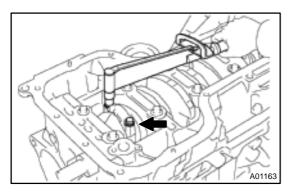
(g) Install the connecting rod cap with the 2 bolts (See page EM-82).
